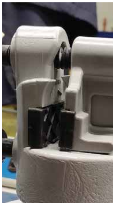
Figure 6-6: [REDACTED] - Typical Insulator Condition after Slip Test (no damage)
