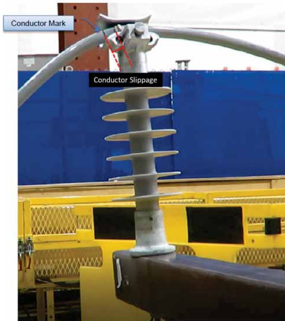
Figure 72. A representative post-test image of a clamp-top insulator tree-fall test (35-kV 1/0 ACSR).
