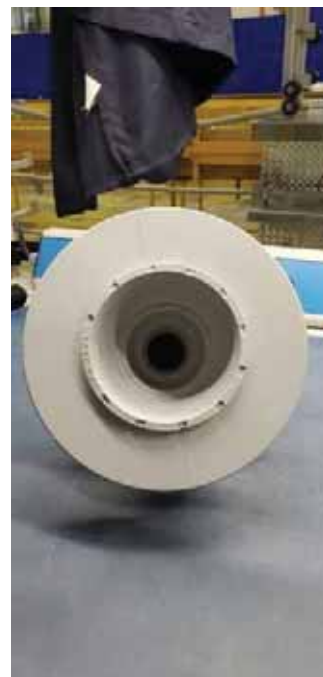
Figure 6-6: [REDACTED] - Typical Insulator Condition after Slip Test (no damage)
