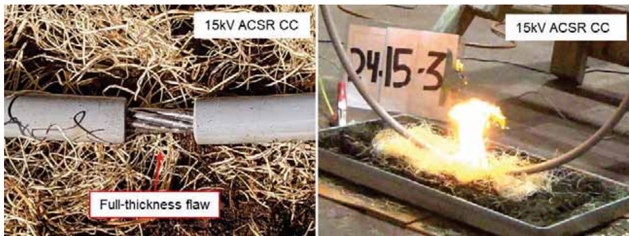
Figure B7. Simulated wire-down test of a 15-kV ACSR CC with a full-thickness flaw demonstrating the potential for ignition of the dry brush.
