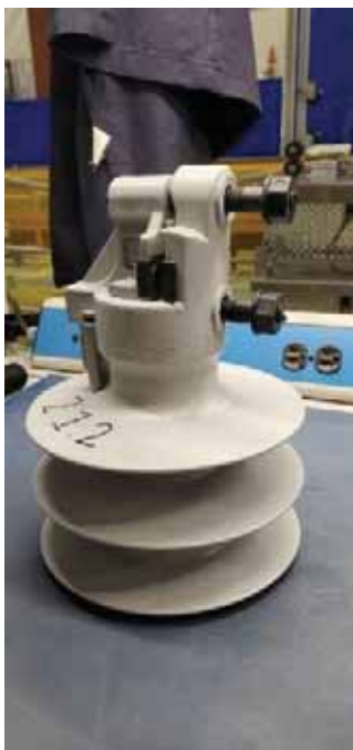
Figure 6-6: [REDACTED] - Typical Insulator Condition after Slip Test (no damage)
