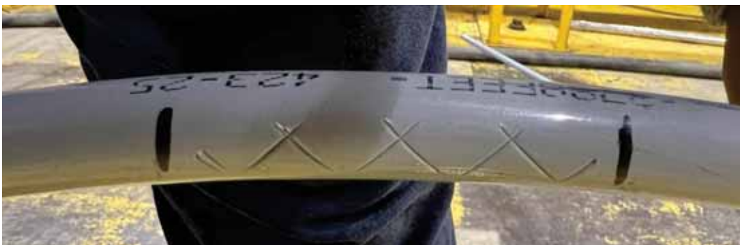
Figure 6-12: Sample 3.1.3 - 17 kV, 1/0 AWG ACSR Condition after Test
