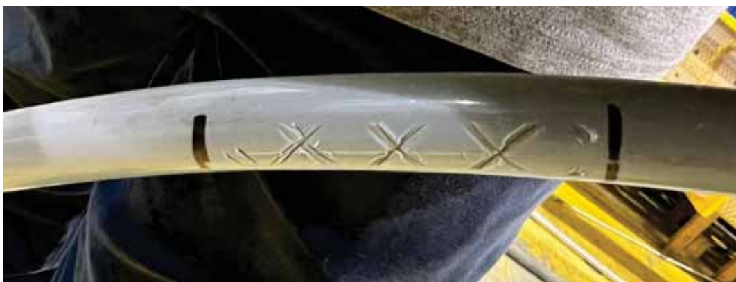
Figure 6-10: Sample 3.1.2 - 17 kV, 1/0 AWG ACSR Condition after Test
