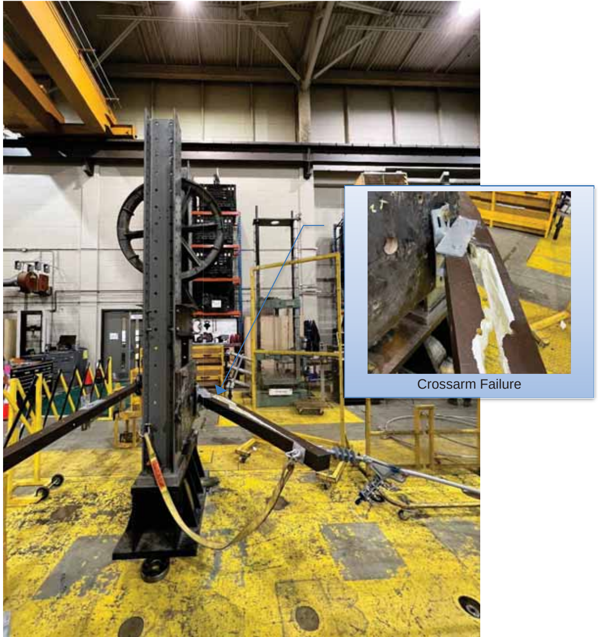
Figure 6-22: Sample 6.1 – Failure Location
