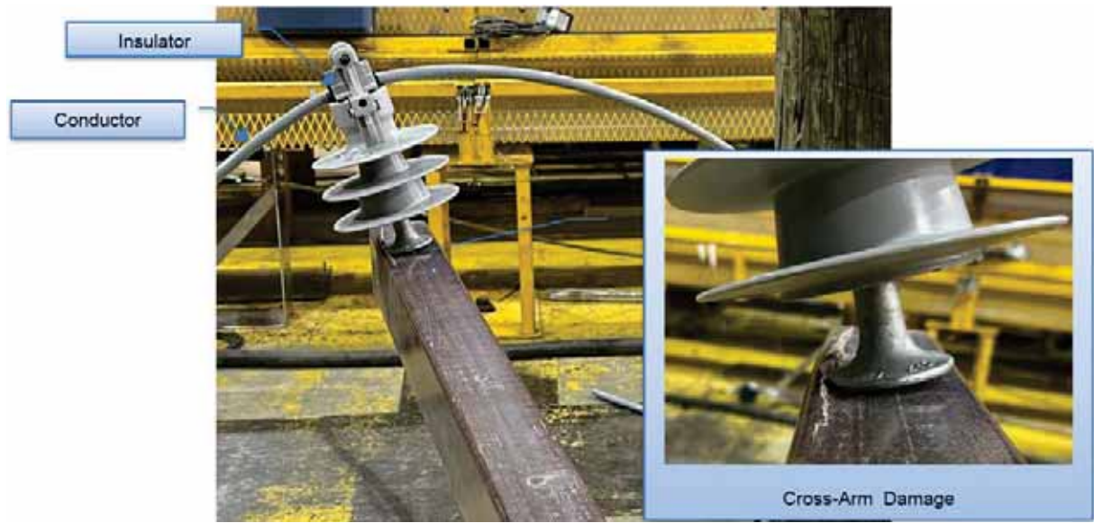
Figure 70. A representative post-test image showing insulator deformation and damage to the cross-arm at its connection point (35-kV 1/0 ACSR).
