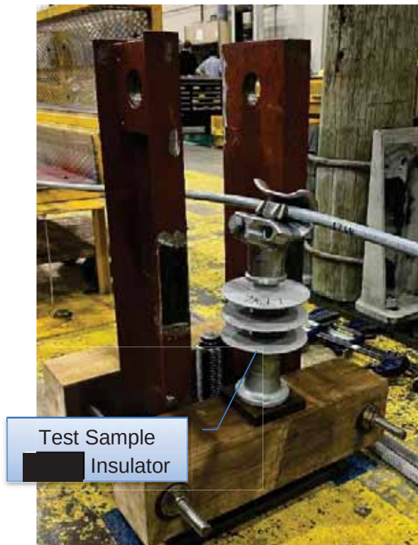
Figure 4-2: Clamp Slip Test Setup
