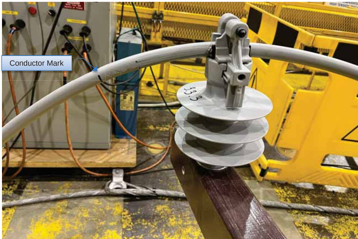
Figure 6-19: Sample 3.3.3 - Insulator and Cross-arm Condition after Test
