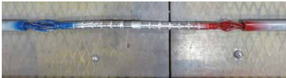
Figure 3-3: █████ installed on 35 kV 1/0 AWG, 6/1 ACSR
