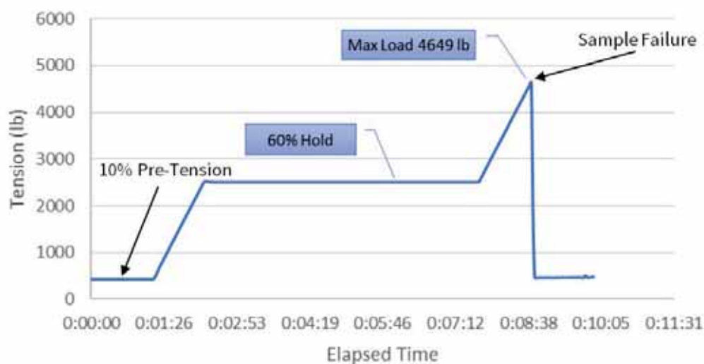
Figure 59. Representative load vs. time plot for the splice maximum load test (Test 1.1).
