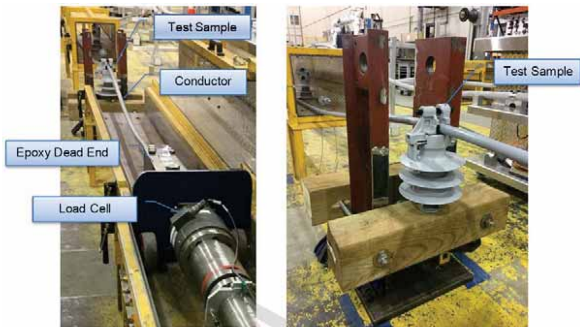
Figure 61. Representative photos of insulator slip test.
