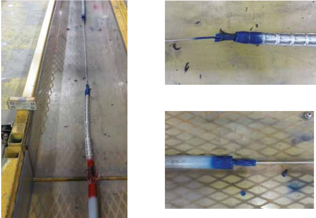
Figure 6-9: Sample 1.2.2 after test (conductor failed at North end of splice)
