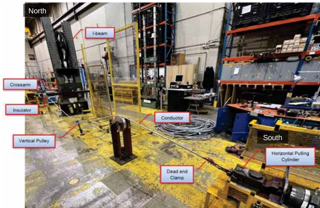
Figure E2. A representative photo of the dead-end tree fall test.
