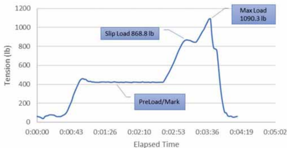
Figure 62. Representative load vs. time plot for the insulator slip test.
