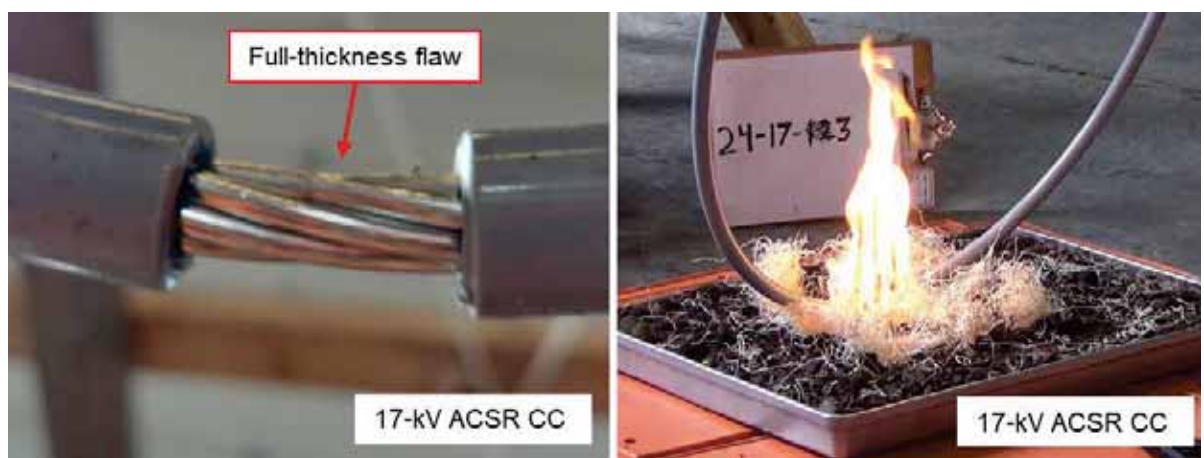
Figure 24. Simulated wire-down test of a 17-kV ACSR CC with a full-thickness flaw demonstrating the potential for ignition of the dry brush.
