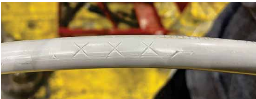
Figure 6-24: Sample 3.4.3 - 15 kV, 1/0 AWG ACSR Condition after Test
