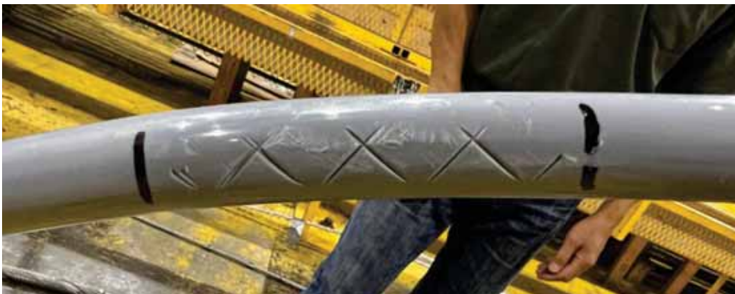
Figure 6-8: Sample 3.1.1 - 17 kV, 1/0 AWG ACSR Condition after Test
